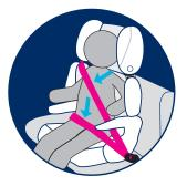
The belt must run through the upper anchorage of the backrest and over the outer part of the shoulder (not touching the neck). The horizontal band must restrain the child by the pelvis (not the abdomen).
