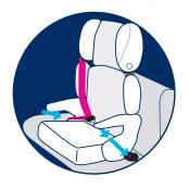
Loose belts or placed under the armpit are the most common examples of misuse in child restraints with belts.
